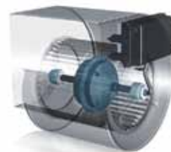
DDMP Scroll casing with direct drive and forward curved blades - double inlet integrated electronics
